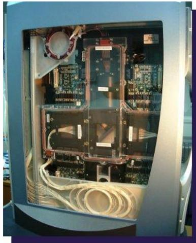
Fig 1. Front view of mounted 64x64 OSM. Input fibers are seen in the lower part of photograph and output are in the upper part. Folding mirrors are seen at the center window
