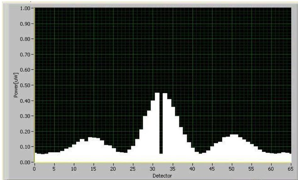
**Figure 1:** Interference pattern for at the output of the channelizer following active phase control at  $f(RF) = 1GHz$
