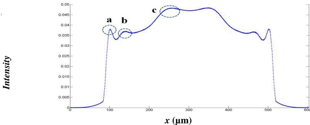
Fig. 2. Three types of filamentation are visible:  $a$ ,  $b$  and  $c$  are 1<sup>st</sup> order, 2<sup>nd</sup> order and 3<sup>rd</sup> order filaments (respectively).
