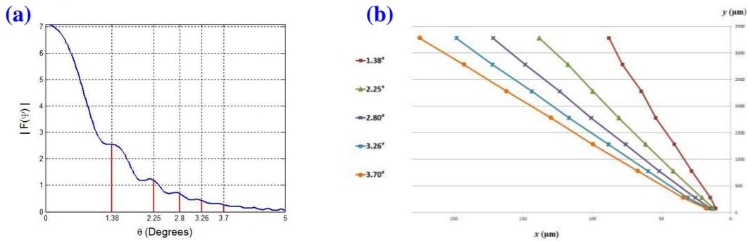
Fig. 4. (a) The Fourier transform of the electric field distribution at the ridge output (a.u.), (b) the ripples in the intensity distribution propagating in a homogenous non-amplifying space. The parameters are the same as in Fig. 3a, except that, in fig. (b), there is no current in the taper section.
