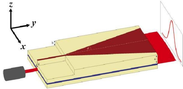
Fig. 1. Schematic diagram of the device. In dark red: p-electrode.  $\theta$  is the half taper angle.  $a$ ,  $b$  and  $c$  are the ridge height, etching depth, and ridge width (respectively). The ridge height, a constant value, is measured from the core to the top of the ridge.
