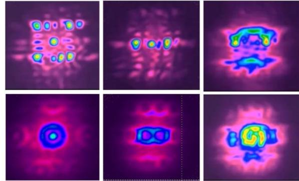
Civan's products and technology allow unlimited beam shapes, by electro-optically manipulating the phases of individual channels. This allows the user to immediately implement advances in research and remain at the forefront of laser material processing, at no additional cost. As there is no need to replace modules, the beam can be shaped during processing, reducing processing time further and allowing for advanced manufacturing techniques.
